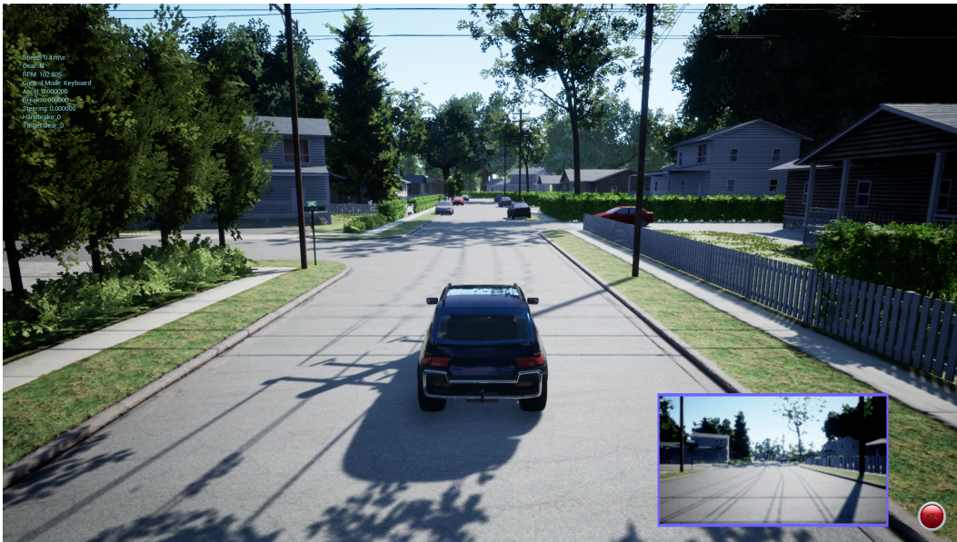
Figure 5: AirSim simulator environment used for our autonomous driving experiments. The egocentric camera view displayed on the bottom left serves as the observations for the autonomous driving agent.
