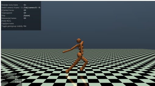
Figure 7: Humanoid Locomotion: A bipedal locomotion task where a simulated humanoid robot must maintain balance and walk as fast as possible (along the x-axis).
