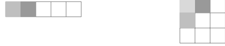
Figure 5: Graphical representation of half kernels used for neural sum layers in layered PNCs. On the left we see a kernel used for one-dimensional data while on the right we have a 3 \times 3 kernel for two-dimensional data. The gray blocks indicate the learnable parameters of the half kernels , while a white square indicates a parameter fixed to zero. Effectively, the convolutional layer is blind with regard to the inputs for these zero elements of the kernel.
