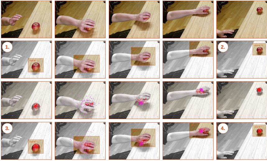
Figure 8.4: A depiction of how suggested system benefits of combined object anchoring and probabilistic object tracking. Rows in order from the top: 1 st ) representing screenshots of a scenario where a human hand is occluding an apple while the apple is moved, 2 nd ) corresponding resulting anchored objects while only using the anchoring system (note that the original apple-1 object is lost while it is occluded and moved by the skin-1 object, and a new apple-3 object is, therefore, acquired in the end of the scenario), 3 rd ) plotted particles given by the inference system during execution of suggested integrated approach, and 4 th ) corresponding resulting anchored objects of the anchoring system supported by the feed back of the inference system (note that in this case is the position of apple-1 object tracked while it is occluded and moved by the skin-1 object, and the apple-1 object is, accordingly, re-acquired in the end of the scenario).
